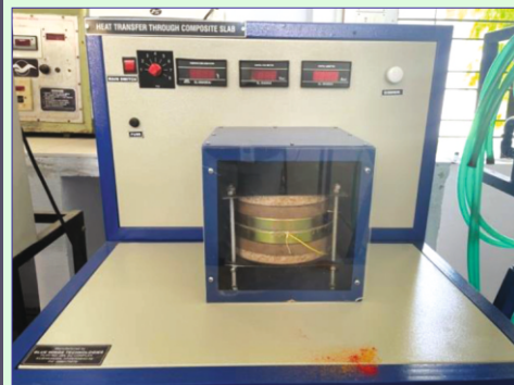
Procured and installed Heat Transfer Laboratory Equipments : (1) Composite walls Apparatus (2) Lagged pipe Apparatus (3) Thermal Conductivity of Insulating powder (4) Thermal Conductivity of metal bar (5) Pin - fin apparatus (6) Unsteady state of Heat Transfer (7) Forced Convection (8) Natural Convection (9) Parallel & Counter flow Heat Exchanger (10) Emissivity (11) Stefan Boltzmann constant (12) Condensation (13) Critical Heat flux and (14) Two phase Heat transfer on 8th April 2022. Total expenditure is Rs. 5,40,000/-
